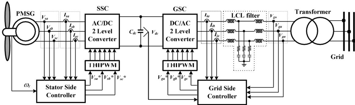
Figure 1. Model of VSWT-PMSG with control system.
