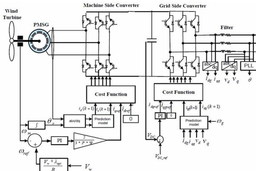
Figure 4. PMSG wind energy conversion system configuration.
