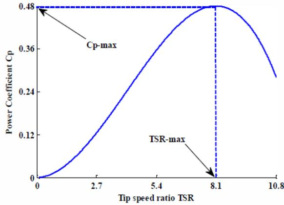
**Figure 5.** Power Coefficient ( $C_p$ ) vs. Tip Speed Ratio ( $TSR/\lambda$ ).
