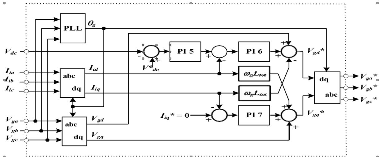
Figure 3. Grid side controller system.
