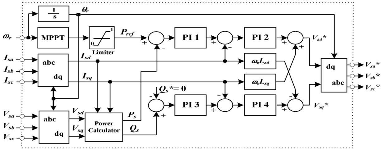
Figure 2. Stator side controller system.
