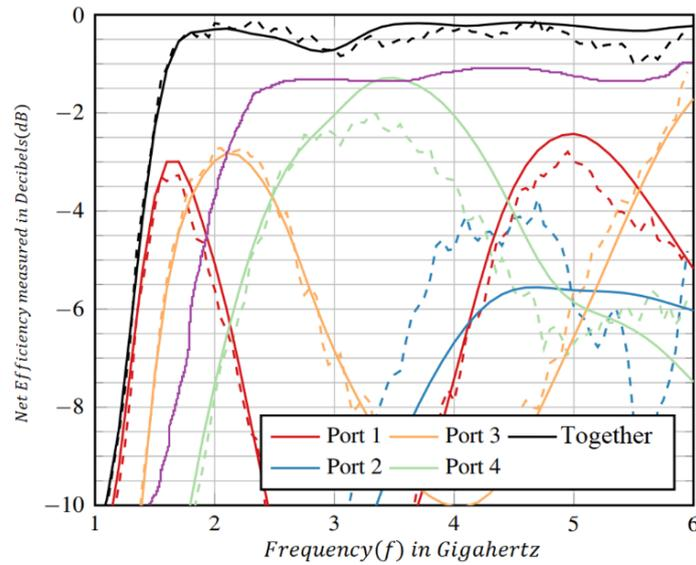
**Figure 6.** Values of efficiency calculated over the 4 ports of the antenna, The solid lines represent the experimentally derived values and the dashed lines represents the simulated values.
