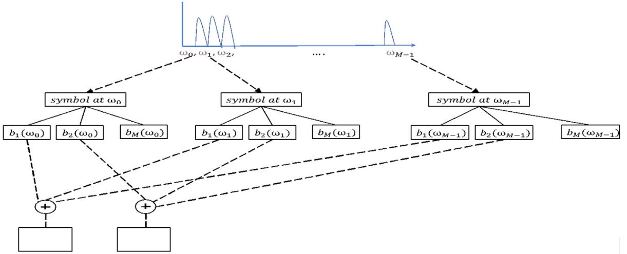
**Figure 2.** The weight of every carrier is done one by one in order to get the system operating over multiple bands, adding these values and transferring them to the input ports of the antennas.
