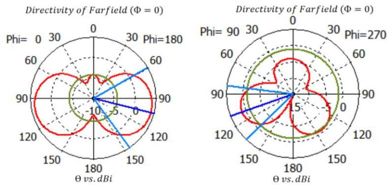
**Figure 8.** (a) Pattern of Radiation at 2.1 Gigahertz for  $\phi = 180$  degrees; (b) Pattern of Radiation at 2.1 Gigahertz for  $\phi = 270$  degrees.
