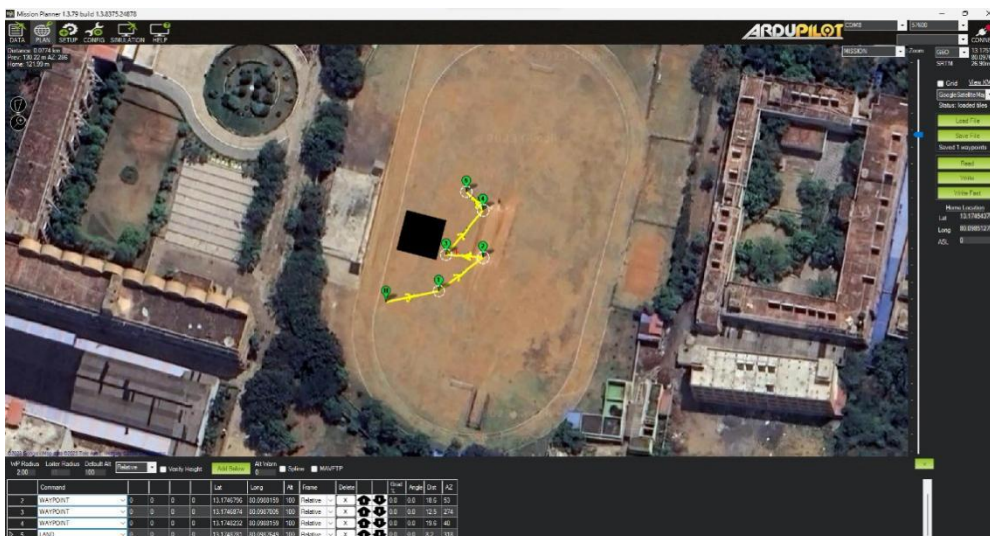
Figure 2. Inducing RRT algorithm in Mission Planner software for obstacle avoidance.
