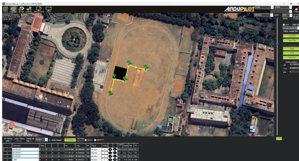
Figure 1. Inducing G-BFS algorithm in Mission Planner software for obstacle avoidance.
