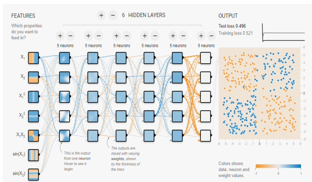
Figure 13. (G) depicts data analysis on seven inputs ( X_1 , X_2 , X_1^2 , X_2^2 , X_1X_2 , \sin(X_1) , \sin(X_2) ) neurons five sets of neurons, six hidden layers with noise [Different data set]
