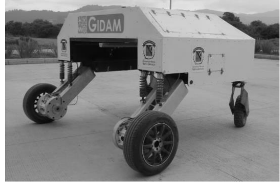
Figure 1. CERES pictures: Electric differential tractor (48V), carrying capacity of 100 kg solid fertilizer, 20 liters fumigation and weeding system.
