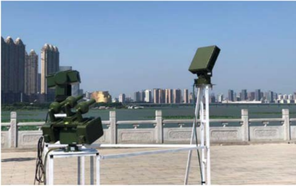
Figure 7. UAV intrusion detection equipment building platform.
