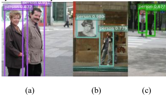
Figure 1. (a) Pedestrian in small pixel is more likely to be missed. (b) Overlapped pedestrian is to be missed. (c) Objects similar to pedestrian appearance are easy for an error detection.
