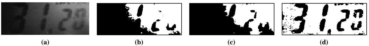
Figure 1. Thresholding of grayscale image: (a) original image; binary image resulting from (b) global; (c) Otsu and (d) local thresholding.
