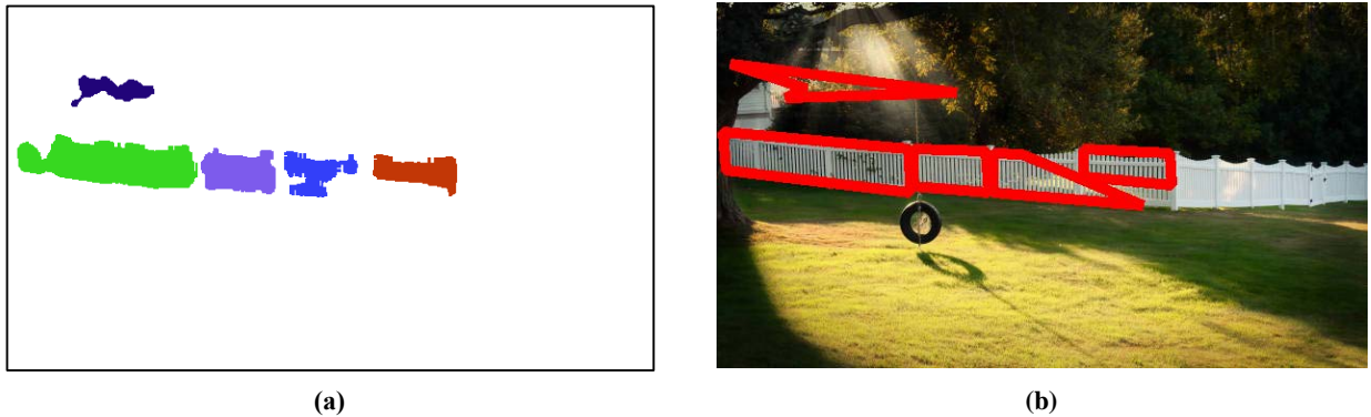
Figure 11. Connected component localization by quadrangles: (a) connected components shown in Figure 6b , after filtering of small area components; (b) fence fragments localization by quadrangles (see Figure 3a ) as the regions of an image with high intensity oscillation level.
