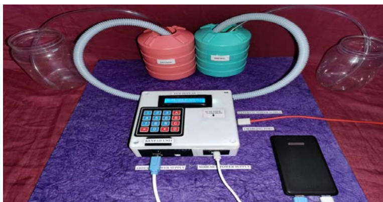
Figure 9. Experimental setup of the automated petrol station.
