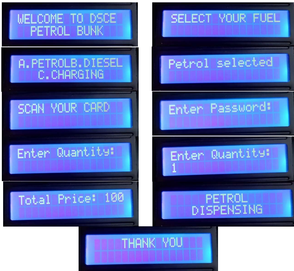
Figure 10. RFID processing steps.
