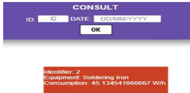
Figure 9. Visualization of electricity consumption in test with Soldering Iron.
