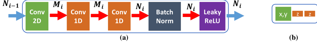
Figure 4. (a) The inner structure of the factorized version of a single 3D convolution; (b) The symbolic representation of the factorized version of a single 3D convolution, where the green square represents a 2D convolution with a kernel size of k \times k \times 1 in x and y coordinates, while each orange rectangle represents a 1D convolution with a kernel size of 1 \times 1 \times k in z coordinates.
