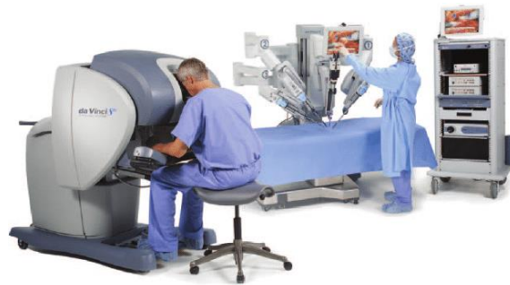
Figure 6. Da Vinci S HD robotic system (surgeons console, patient side card with robot arms, InSite Ö vision system) (a [2008] Intuitive Surgical, Inc.).
