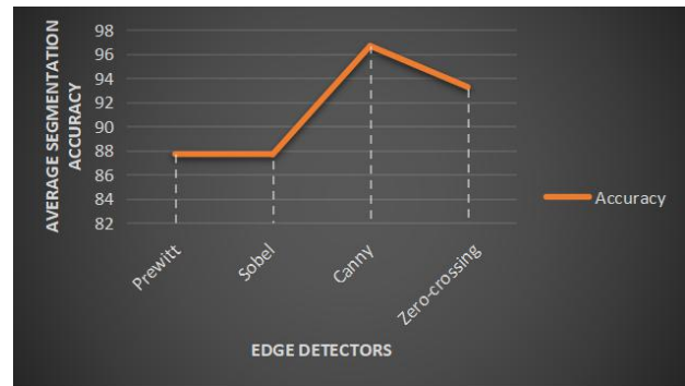
Figure 4. Comparison the average segmentation accuracy based on proposed method BiltSp-Poly using different edge detectors.
