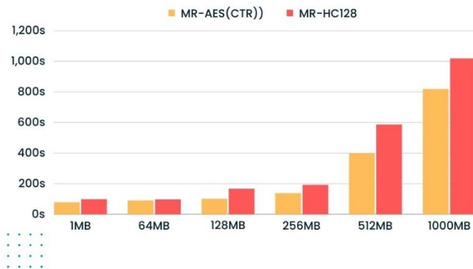
Figure 6. Encryption time AES(CTR) Vs HC-128.
