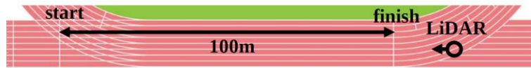
Figure 5. The experimental environment where point clouds were acquired. The distance from the start line to the finish line was 100 m. The LiDAR was installed facing towards the start line and placed behind the finish line.
