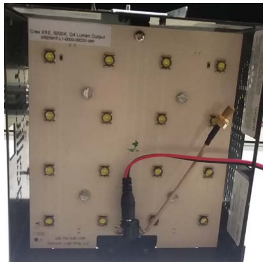
Figure 1. The underside of a tracking fixture unit. Infrared receiver not included.
